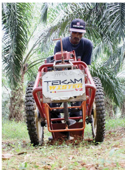
Mechanisation equipment such as Tekam Twister, a subsoiler for fertiliser manuring improves productivity significantly.
