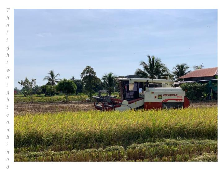
harvester is used to prevent damage on hardpan soil
